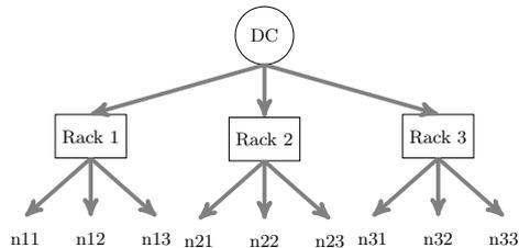
The probability that the entire DC breaks down (e.g., in a disaster) is  $1/20$ , the probability that a specific rack (switch) breaks down is  $1/10$ , the probability that a specific node breaks down is  $1/4$ . For simplicity, we assume that the probability that a failure happens is independent of other failures.
